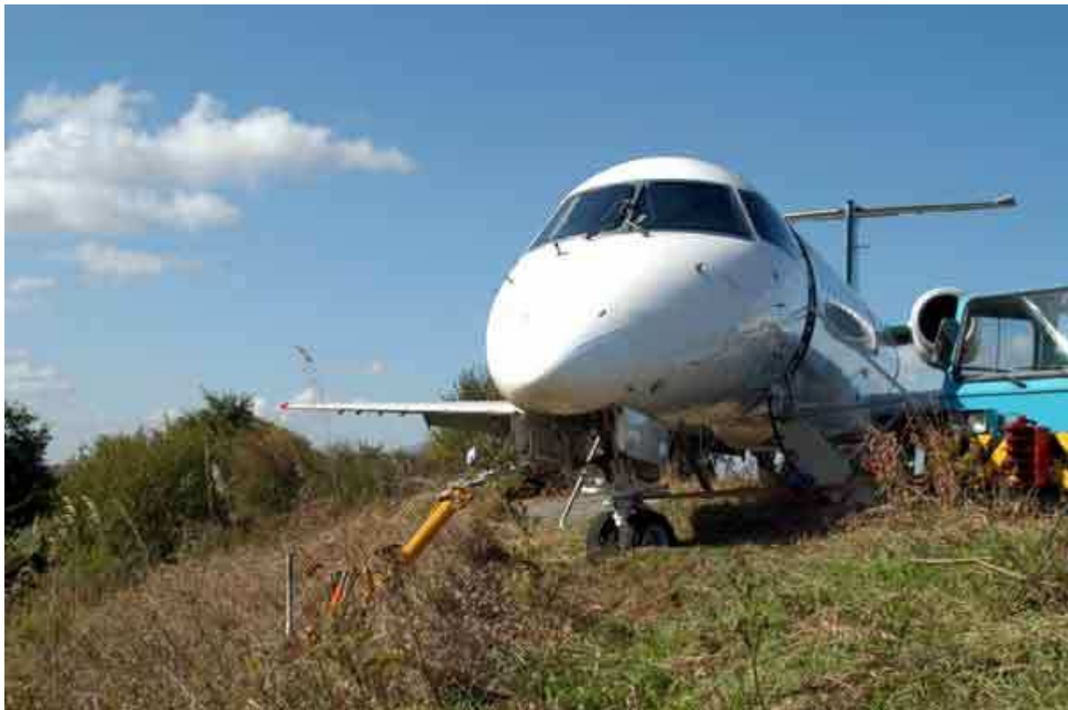
EMB-145 veered off the runway after landing due to nose wheel steering problems (23-9-2003, Luxembourg).
