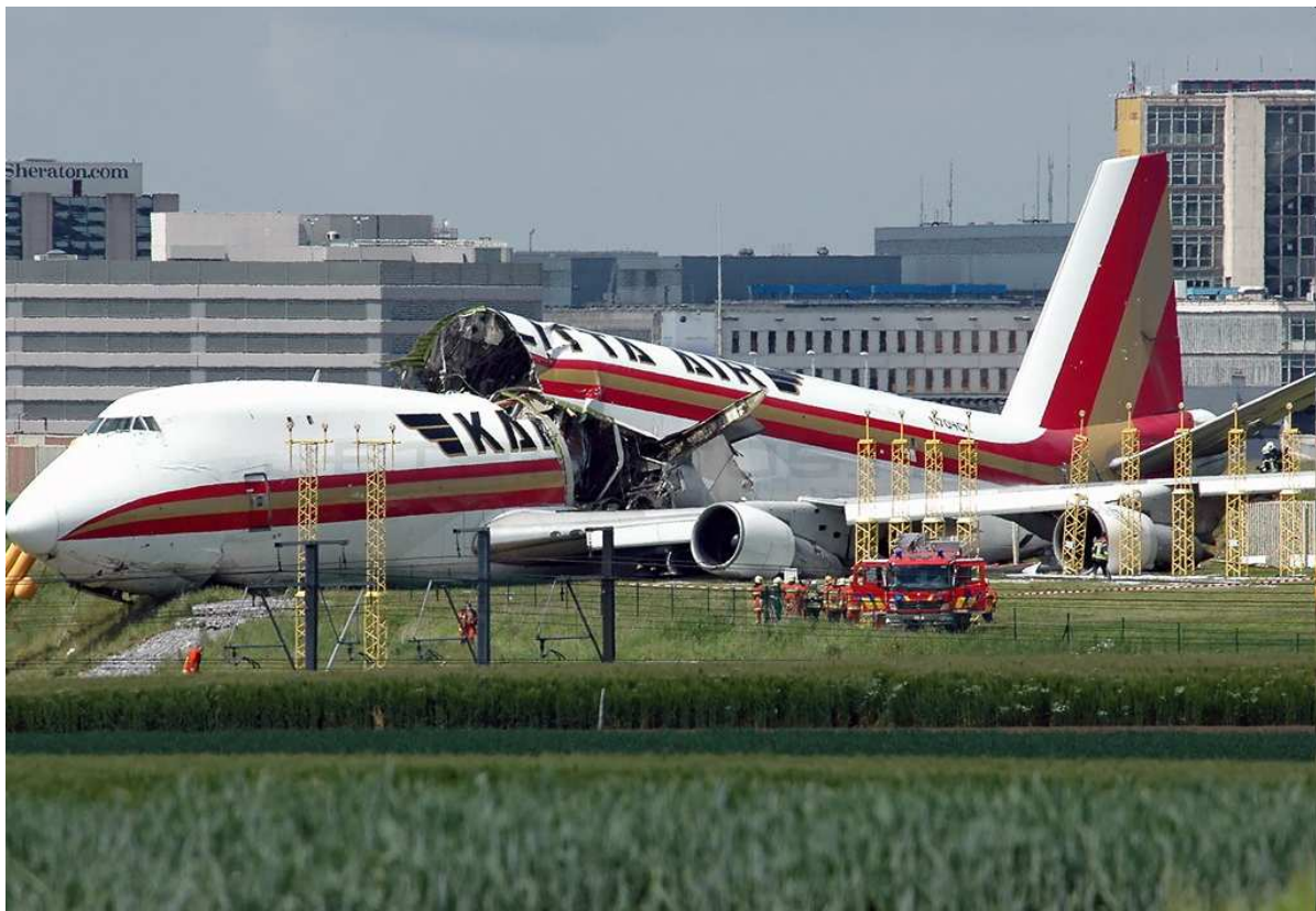
Overrun of a B747-200 after a high speed rejected takeoff (Brussels Airport, 25-May-2008).
