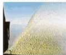
SLD - Total coverage of the unheated part of the side window. The yellow color is due to the water used during tanker tests.
