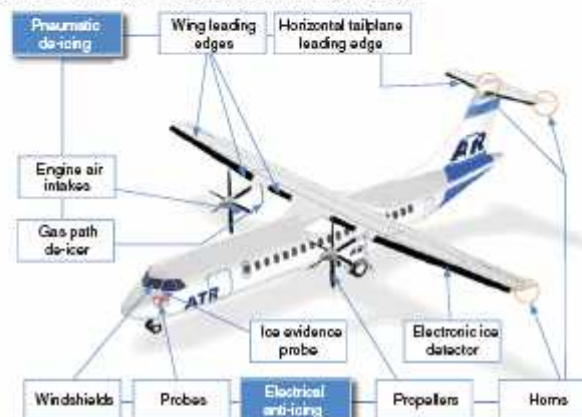
Example of ATR 72-500 basic ice protection system
