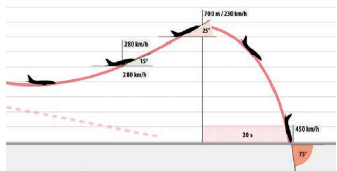
Tatarstan 363 (B737-500) Go-around and crash profile. FlyDubai 981 profile almost identical!
