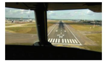
Of course, the risk could be compounded with a malfunction of an aircraft system such as the brakes or spoilers. The runway conditions also can have a detrimental effect with a runway contaminated with standing water inducing aquaplaning with a resulting loss of directional control.
