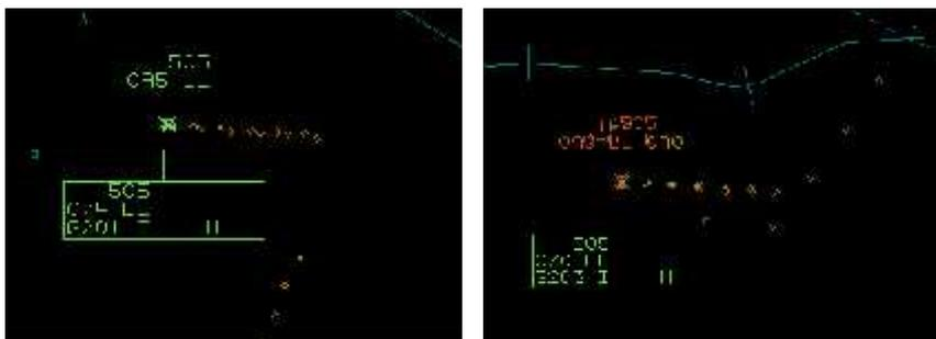
Figure 2 - Splits and Corruption in the Lamborne Stack. One aircraft is detected as two with the same identity (505) but corrupt and different heights this then leads to a false conflict alert with a second non existent aircraft, that results from a subsequent corruption of identity (505->168) –this would not have occurred in the Mode S pattern.
