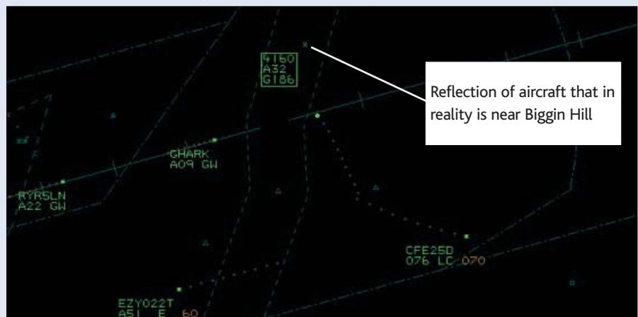
Figure 2 - Splits and Corruption in the Lamborne Stack. One aircraft is detected as two with the same identity (505) but corrupt and different heights this then leads to a false conflict alert with a second non-existent aircraft, that results from a subsequent corruption of identity (505->168) – this would not have occurred in the Mode S pattern.
