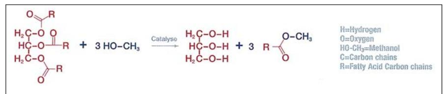
Figure 1: Example of the FAME manufacturing process by transesterification
