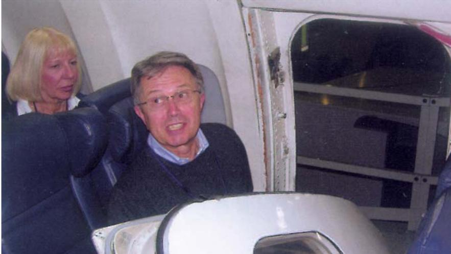
*The overwing exit doors weigh 40 lbs and must be thrown out of the aircraft*
