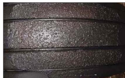
Left: Figure 1 – marks of rubber reversion hydroplaning on the tyre.
