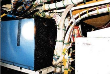
General view, looking forward and outboard, of the aft inboard corner of the galley chiller unit (blue) in relation to the wiring looms. Crew emergency oxygen bottle is located beneath chiller.
