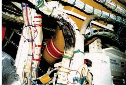
General view of damaged wires after chiller removal, with partially failed loom nearest the camera. Areas identified A and B exhibit wire damage not directly related to the loom failure. Of significance, damage at A is approximately the same height as the failed section of loom.
