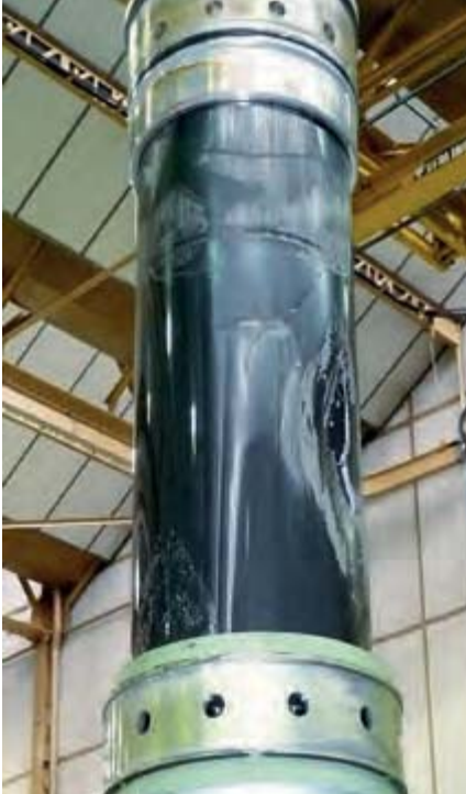
Figure 3: Damage on the aircraft following the hard landing: aircraft's Landing Gear
