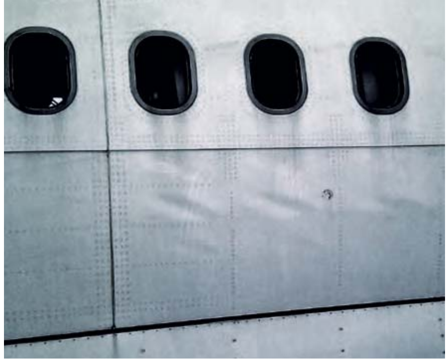
Figure 4: Damage on the aircraft following the hard landing: ripples on the fuselage
