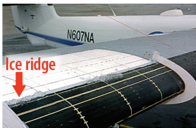
Photo C — Ice ridge on icing research aircraft from a freezing rain encounter, after much of the ice had melted and/or shed after landing
