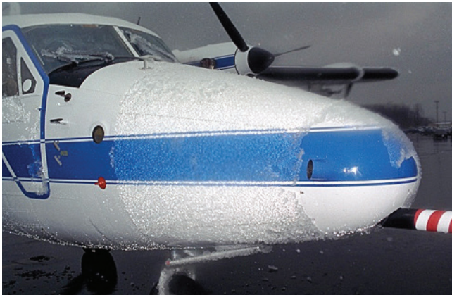
Photo D — Freezing rain formation on the nose of an aircraft from a freezing rain encounter
