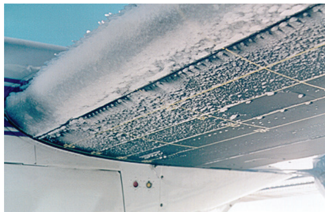
Photo B — Supercooled large droplet formation on unprotected wing
