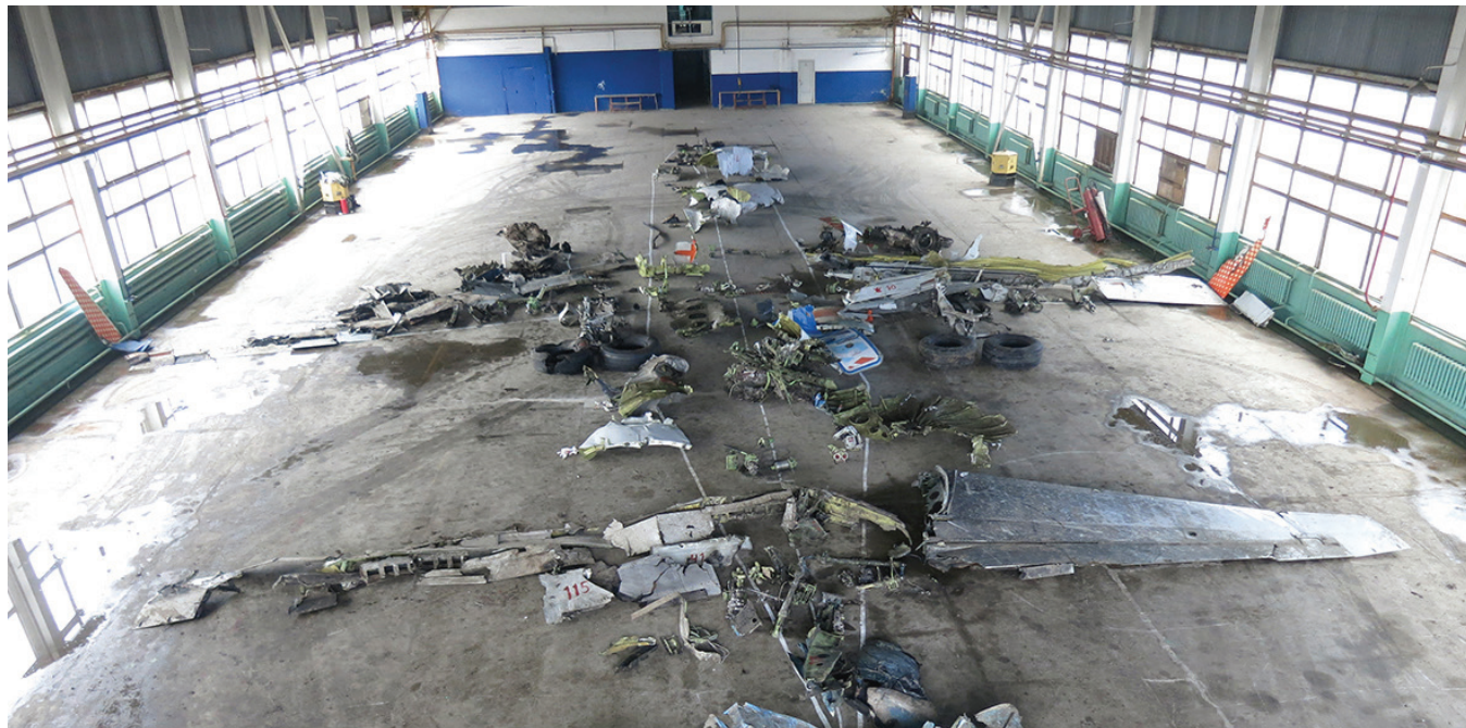
Source: The wreckage of the FlyDubai 737-800 laid out on a hangar floor by investigators. (Photo MAK)
