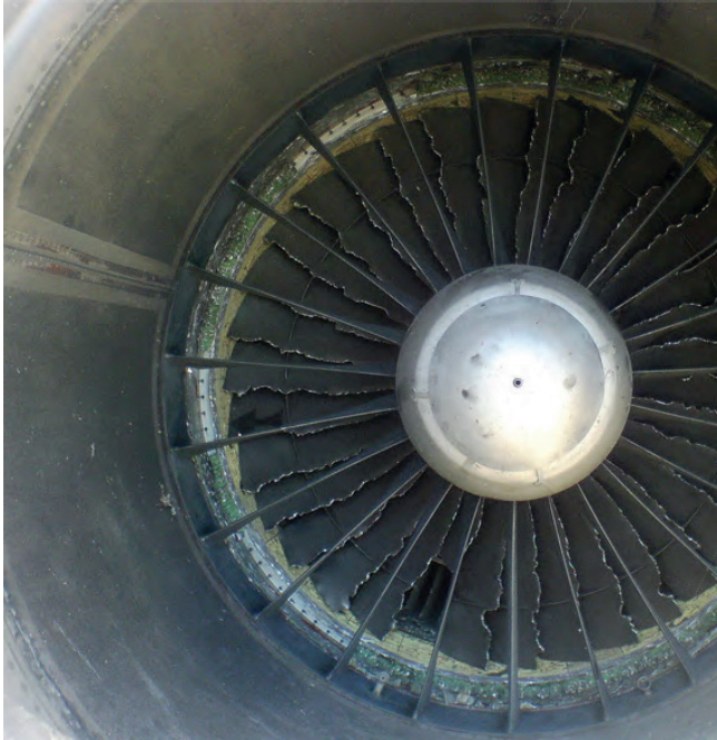
The damaged fan blades of a Pratt & Whitney JT8D engine after a bird strike.
