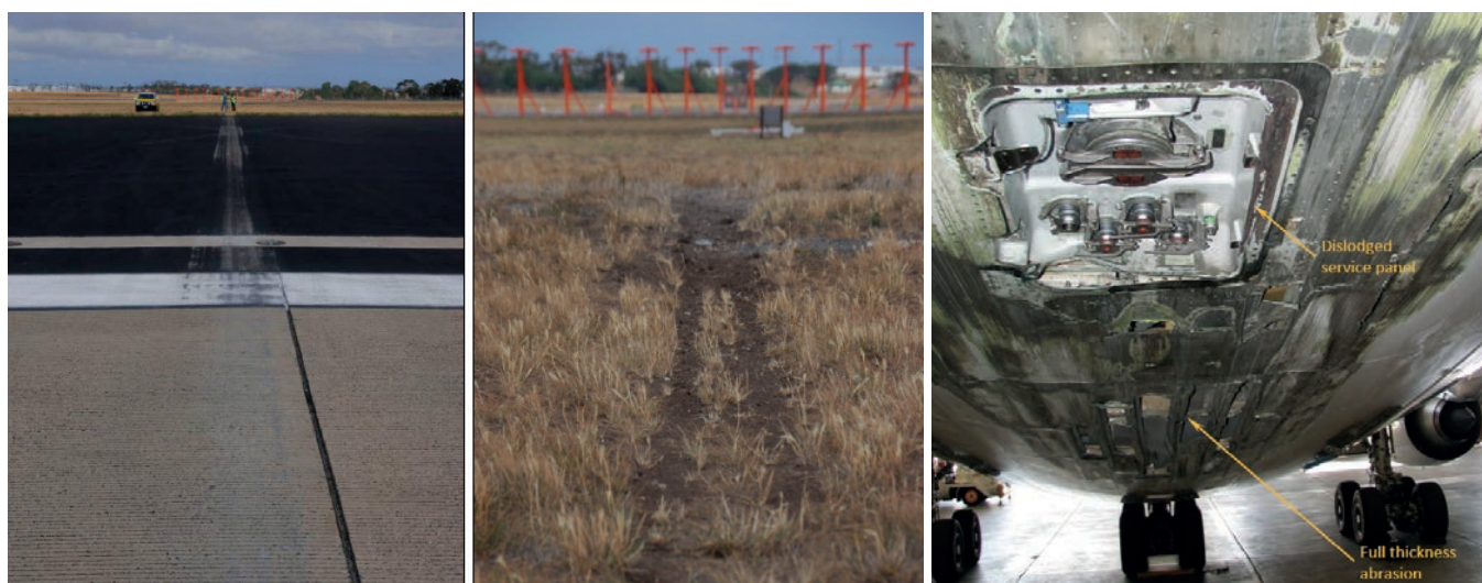
Figure 2 Contact marks on the runway, overrun grass and underside of the aircraft.
