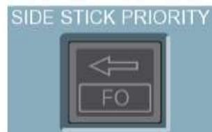
By pressing the button on the side stick, the pilot takes over control as long as he maintains the pressure.
