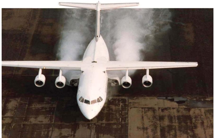
Above: wet runways contamination can cause hydroplaning
