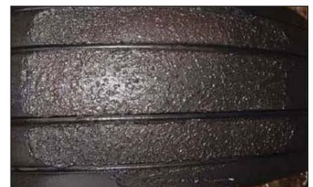
Left: Figure 1 – marks of rubber reversion hydroplaning on the tyre.
