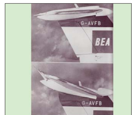
3. Some all moving tailplanes are trimmed conventionally – the Trident's was commanded by both the column and the trim wheel; the 'elevator' was a geared tab (reproduced with permission from CAA)
