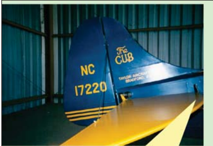
4. Trimming tailplanes aren't confined to the jets – this Piper Cub has one, as shown by the slot near the tailplane leading edge, which provides access to the actuating link
