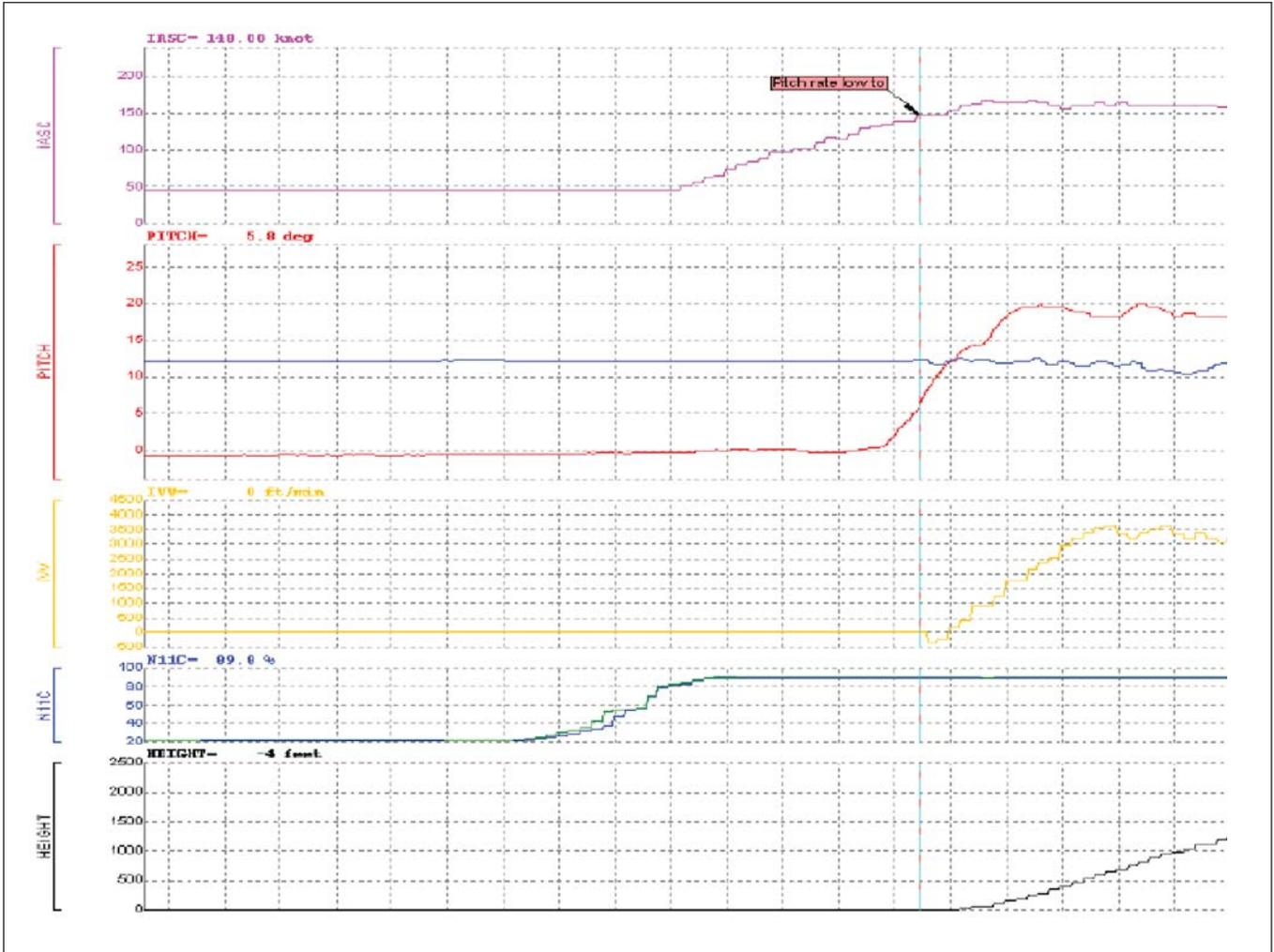
With each rectangle in the graphs representing five seconds the effects of the slow rotation can clearly be seen. When all this data is shown to the crew it becomes a very good tool for demonstrating the errors of their ways and it is important that they fully understand the effects on performance of not operating the aircraft in the correct manner.
