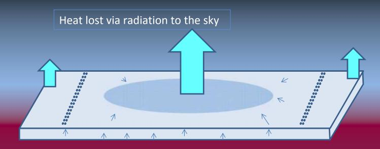
No heat transfer to the air (no temperature differential)
