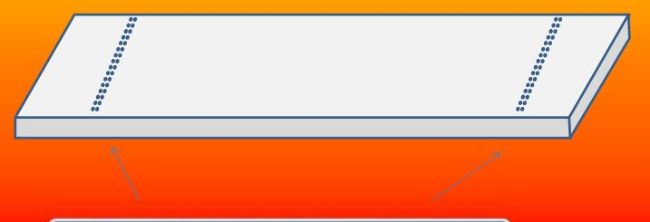
Metal Rivets to supports and actuators
