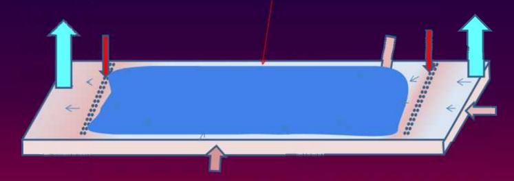
Net Result: frost pattern spreads outward, eventually involving the entire surface Radiation heat transfer is disrupted by the frost layer and the surface temperature stabilizes near the frost point.
