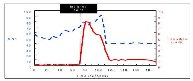
Fan vibration levels should return to normal levels as fan ice sheds
