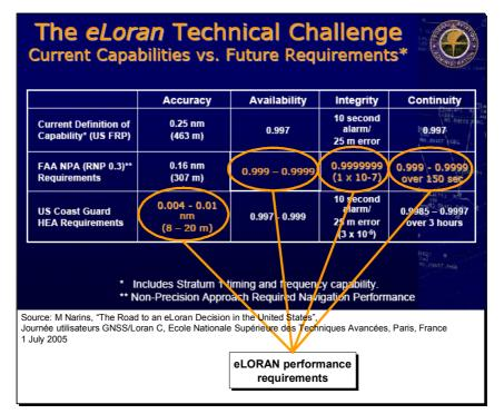
Clearly, this formidable set of requirements exceeds in respect of every parameter the performance standards of traditional LORAN-C. The modernisation of the system that has enabled this higher performance to be achieved is detailed in the set of "eLORAN actions" presented in the tables below. These may be regarded as a checklist of the improvements required to bring the US LORAN-C system up to the new eLORAN standard.
