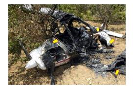
At about 11.00 hrs after flying from Portimão the three axis microlight was on the final approach about 1 km from the landing strip when the pilot dodged a bird by turning and diving. The aircraft struck power lines which became entangled with the aircraft. It crashed 180 metres from the displaced threshold. The two occupants escaped, the pilot suffering a minor arm injury but the aircraft was destroyed by fire.
