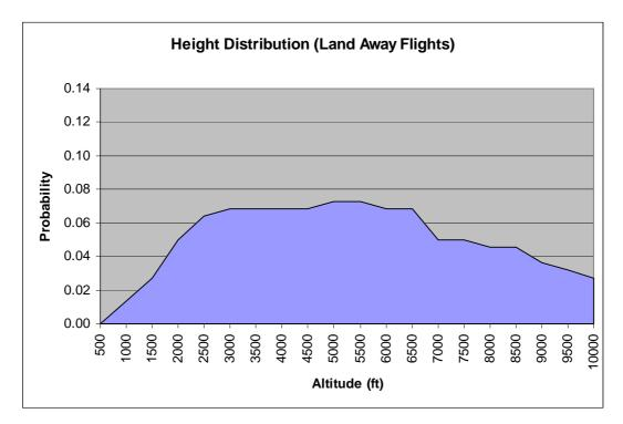
**Observation:** There is a striking difference between local (return-to-base) and land away flights, with the majority of local flights being conducted between 1,500 and 3,500 ft. For land away flights, operation is most likely between 2,500 and 6,500 ft.
