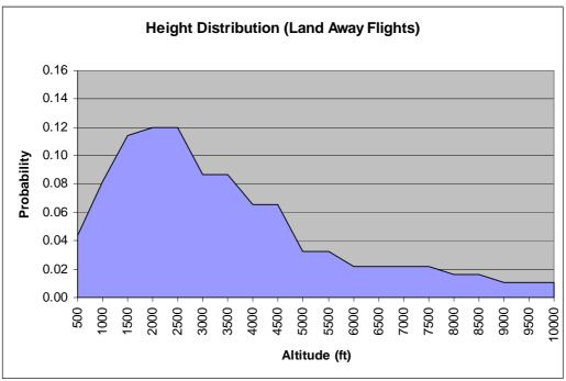
**Observation:** There is very little difference between the above charts. Both show that Flexwing Microlights are most likely to operate below 3,000 feet, The most likely operating altitude for return-to-base flights is 1,500 ft, whereas between 2,000 and 2,500 ft is most likely for land away flights. Perhaps surprisingly, a significant number of users claim to operate at altitudes of up to 9,000 ft.
