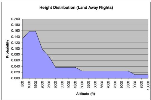
**Observation:** For local (return-to-base) flights that return to the launch site, the most likely operating altitude is around 1,000 ft, and few flights are conducted above 3,000 ft. For 'Land Away' flights, operation at greater altitude is more likely. It is worth noting that 1,500 ft to 2,000 ft is the most popular altitude range for cross-country flights.
