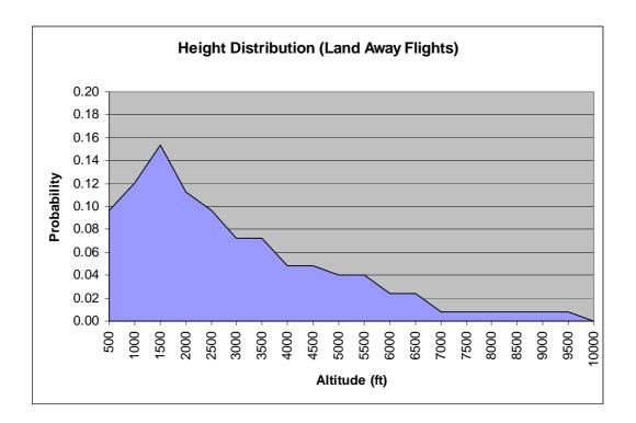
**Observation:** The above graphs suggest that, whilst flights can be conducted at altitudes of up to 10,000 ft, the most likely operating altitude is around 1,500 ft. Cross-country (land away) flights tend to operate at higher altitudes.
