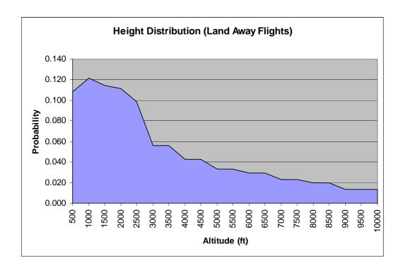
**Observation:** From the above graph it can be seen that the majority of hot air balloon flights are conducted below 3,000 ft. Statistically, 1,000 ft is the most likely operating altitude.
