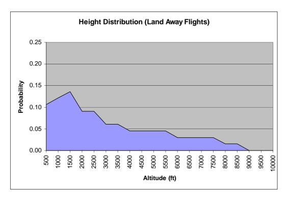
**Observation:** In both graphs, the most likely altitude is between 1,000 and 1,500 ft. For local area (return-to-base) flights, the majority of activity takes place below 2,500 ft, whereas for land away flights, operation up to 8,000 ft is not uncommon.
