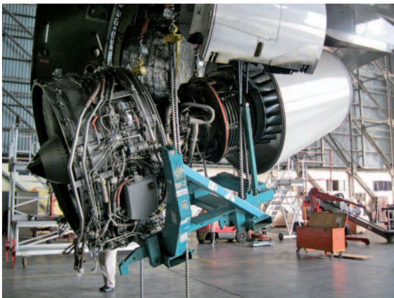
Figure 2 consequence of disengaged chain pulley
