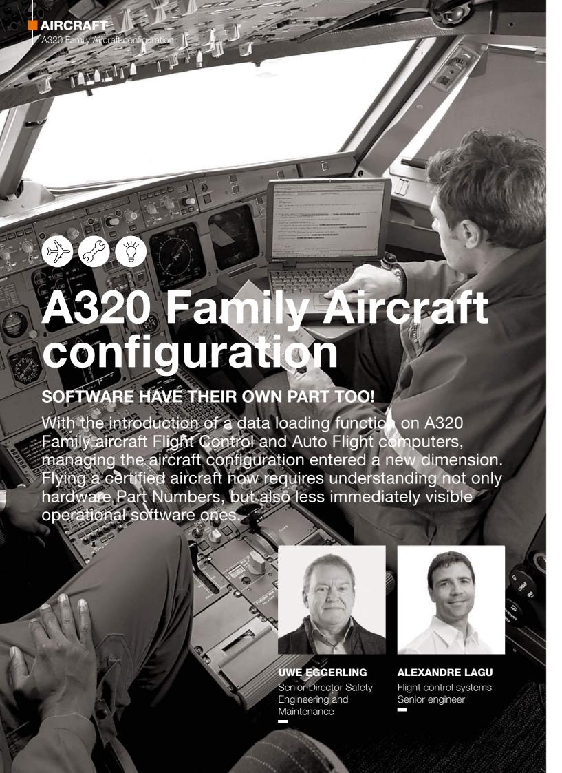
In 2009, a new data loading function was introduced on A320 Family aircraft Flight Control and Auto Flight systems computers. Although the operational improvements brought by Field Loadable Software (FLS) are widely appreciated, experience gained with them highlights a potential for aircraft configuration mismanagement as a result of improper software part number uploading in the computers.
