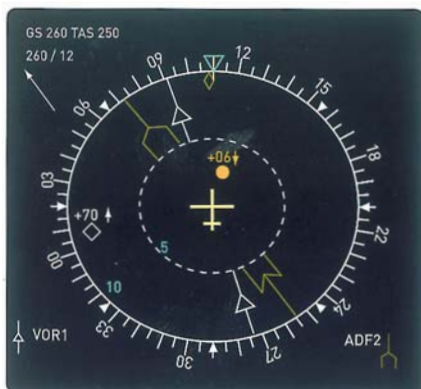
Figure 1: Navigation Display in case of TCAS TA
