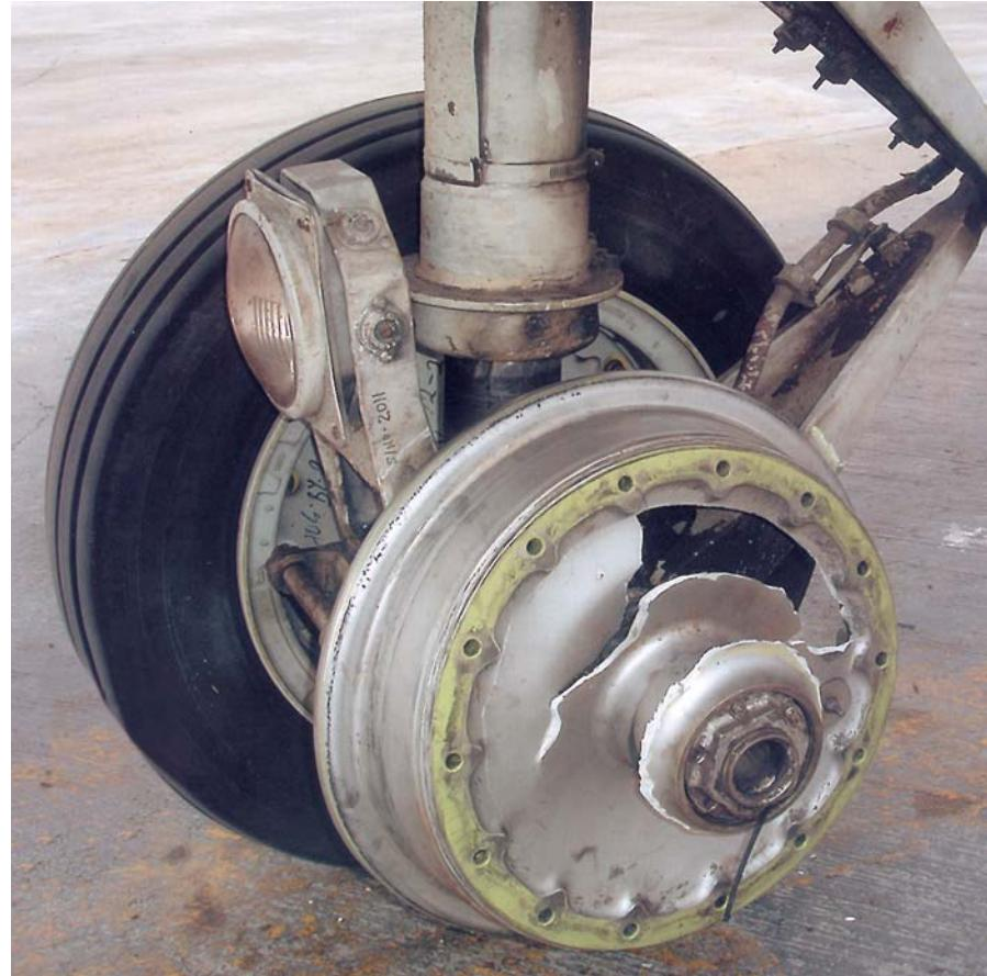
*Figure 1 – Wheel damage due to overinflation*
