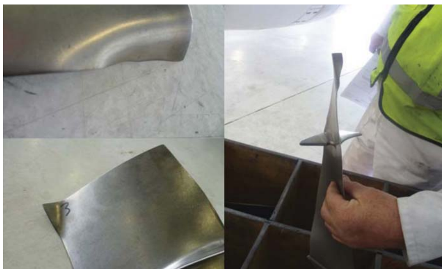
Figure 1: Damage to the fan blades of both engines on SJC
