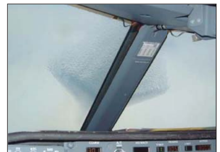
Figure 5: Extensive ice on a heated windshield is a likely indication of severe icing, according to the website: http://www.b737.org.uk/iceandrain.htm
