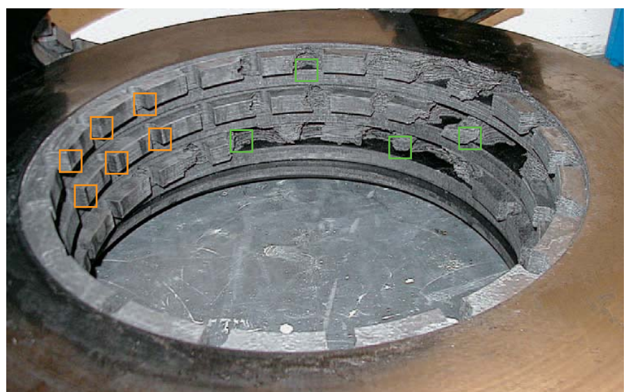
Figure 2: Damage to carbon brake disks caused by runway deicers. The damaged stator disk drive lugs on this carbon heat-sink demonstrate the type of damage alkali metal-based runway deicers can cause to carbon brake disks.
