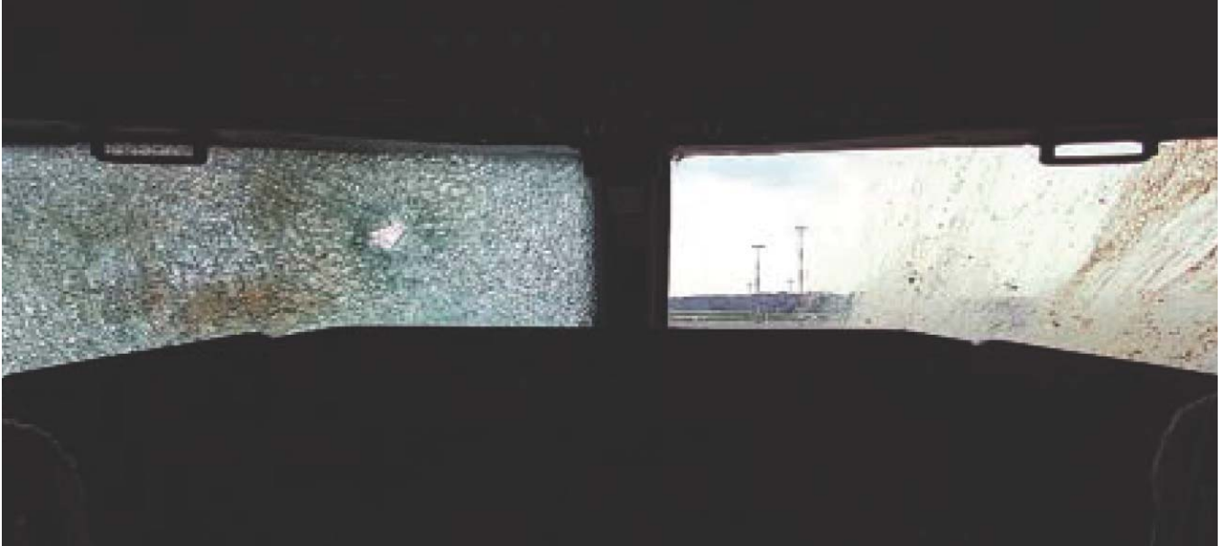
An Air Berlin Boeing 737-700 windshield after encountering a flock of white-fronted geese at about 2,150 ft and 226 kt indicated airspeed.
